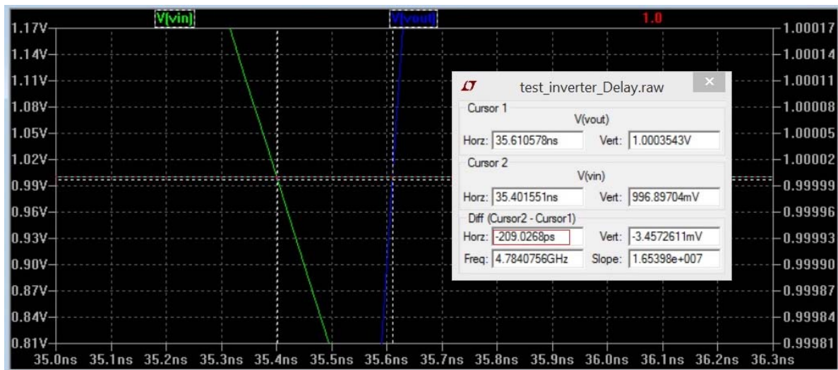
Figure 28. Find t_{pLH} from the graph
