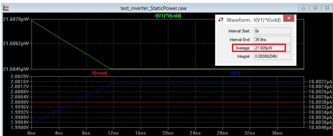
Figure 38. Capture the static power from waveforms
